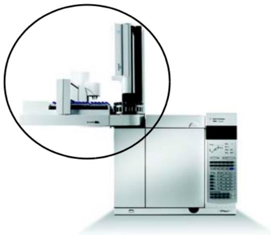
Install the sampler and tray and connect the cables to the back panel.
