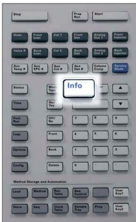
**[Info]** Provides context-sensitive help for the currently shown parameter. For example, if **Oven Temp** is the active line in the display (has a < next to it), **[Info]** will display the valid range of oven temperatures. In other cases, **[Info]** will display definitions or actions that need to be performed.
