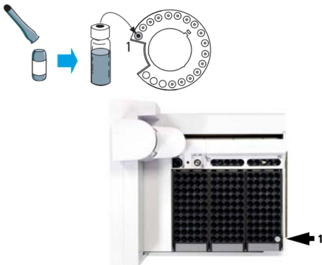
For **automatic sampler injections**: Prepare the checkout sample vial. Load the vial into the sampler, then press start.
