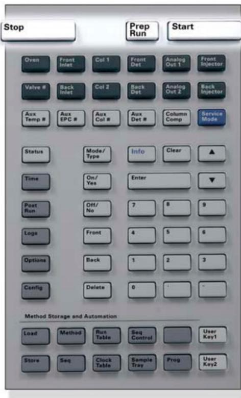
**[Stop]** Immediately terminates the run. If the GC is in the middle of a run, the data from that run may be lost. Refer to the [Agilent 7890A GC Advanced User Guide](#) for information on how to restart the GC after pressing **[Stop]**.
