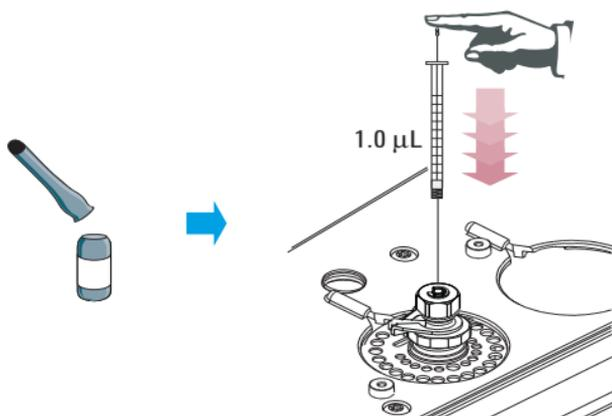
For a **manual injection**: Prepare the checkout sample. Inject the sample into the inlet, then press start.
