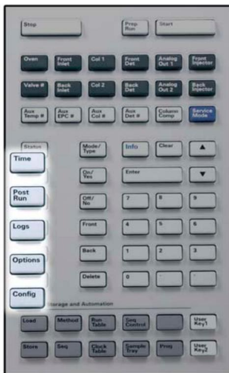
**[Time]** Displays the current date and time on the first line. The two middle lines show the time between runs, the elapsed time and time remaining during a run, and the last run time and post-time during a post-run.
