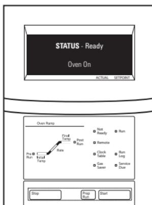
Turn on the GC. Load the checkout method for the inlet and detector you are using. Wait for "Ready" to appear on the display screen.
